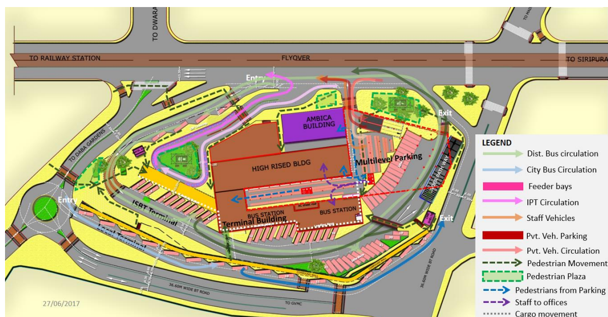
Figure 25: – Design Proposal of Dwarka Bus Station Option 1
