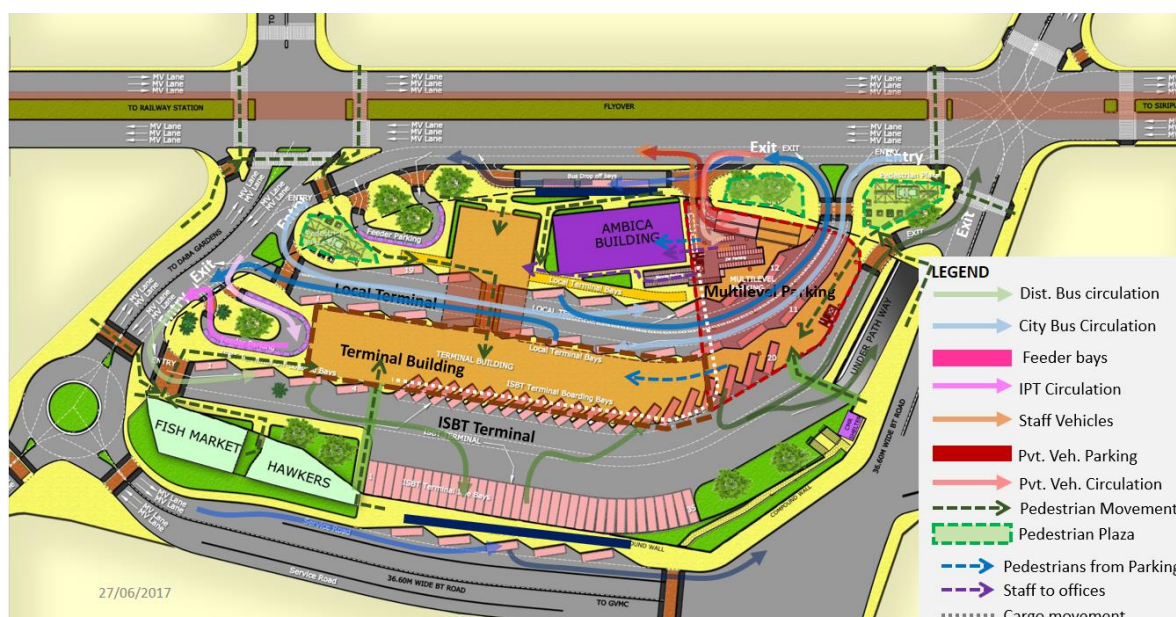
Figure 26: – Design Proposal of Dwarka Bus Station Option 2
